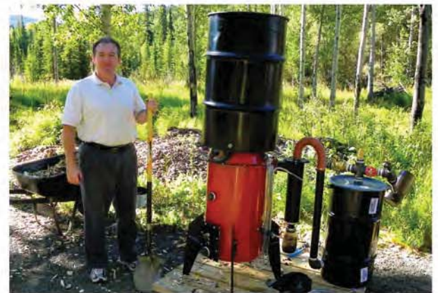
Chena Power's William Bilbow stands with his shovel ready to feed wood chips to our new gasifier. This technology creates hydrogen fuel that can be used to power combustion engines
